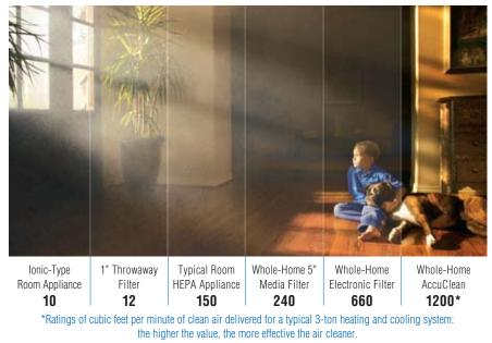
Clean air delivery rate (efficiency times airflow rate) is recognized by the Federal Trade Commission (FTC) and the Environmental Protection Agency (EPA) as a fair and objective measure of various air cleaner technologies.
